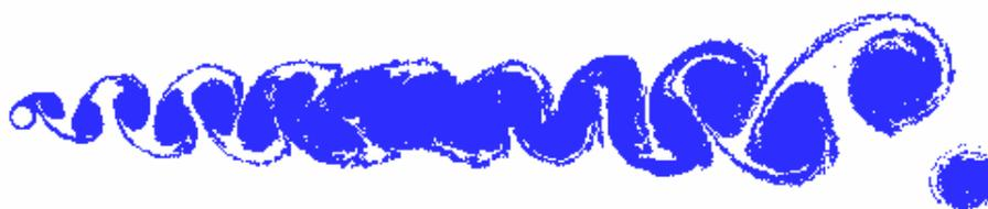
$$A/d=0,15, V_R=5 \text{ e } lock-in: f_0 / f_{s0} = 1$$
