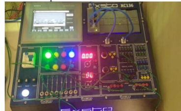
Figure 8. PLC module for controlling the experiment.
