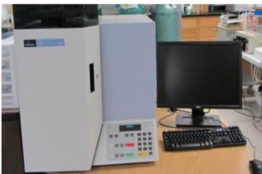
Figura 51: Analisador CHNSO da Perkin Elmer series II 2400. (Oliveira, 2014).
