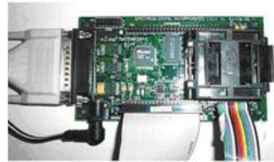
Fig. 5 - Photo of the DSP board development kit
