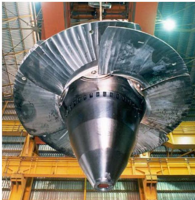
**Figura 25 – Turbina Kaplan**
