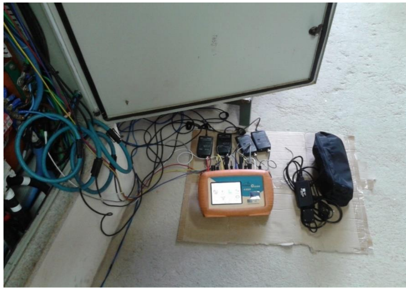
Figure 7.3– PQ Analyser installed in the output of the PV (OLIVEIRA et al., 2015).
