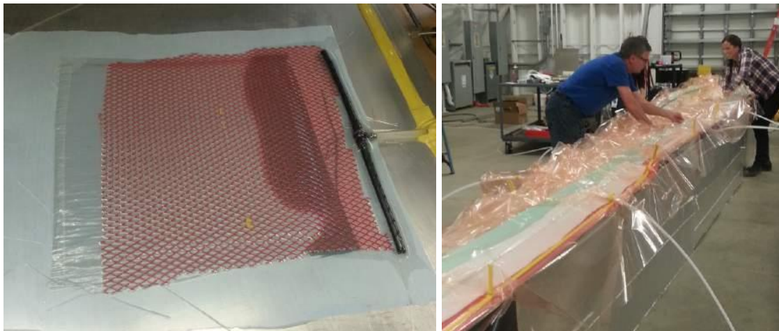
Fig 1.1 - VARTM of a composite test panel (left) and setup of VARTM for infusion of a 13 m prototypical thermoplastic wind turbine blade [15]
