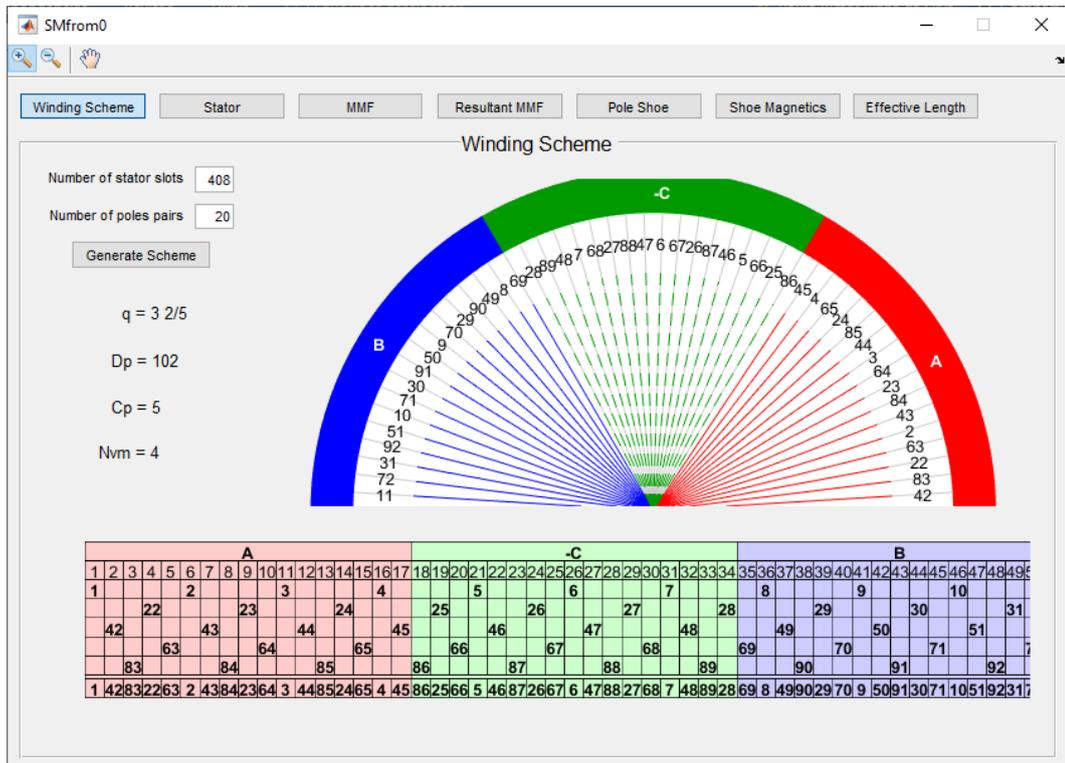
Figure 4.11 - Phasorial rosette and winding scheme for SG2.
