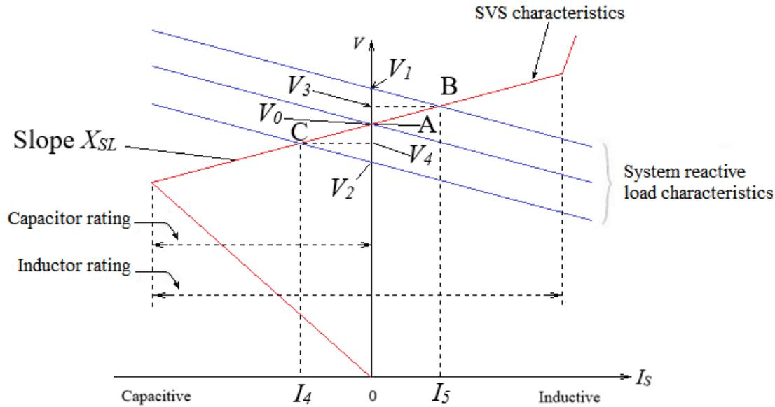
Figure 3.4. – Graphical solution of the SVS point of operation for system conditions.
