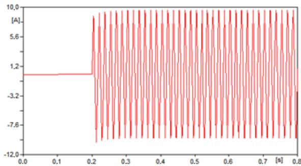
Figure 6.6.5. – Inrush current when energizing the transformer
