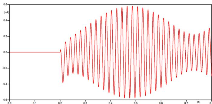
Figure 6.6.4. – Waveform of the harmonic distortion supplied in the inrush current.
