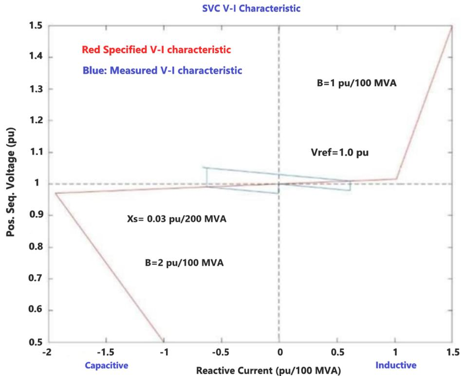
Figure 6.2.3. – Variation of voltage and reactive current.
