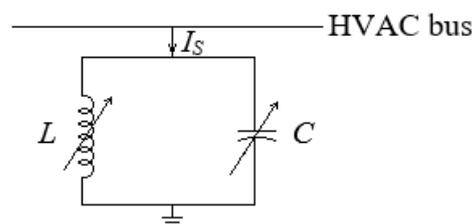
Figure 3.2. – Static var system (SVS).
