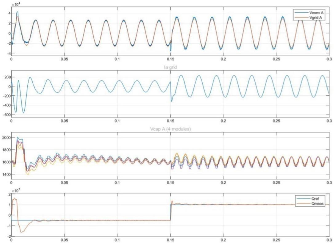
Figure 6.4.3. – Voltages and powers in the statcom.
