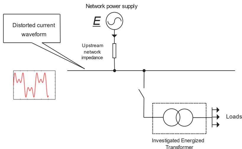
Figure 6.6.1. – The network energy degradation process and the transformer connection network point.
