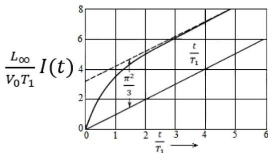
Figure 5.1. – Flux penetration into transformer core under surge conditions.
