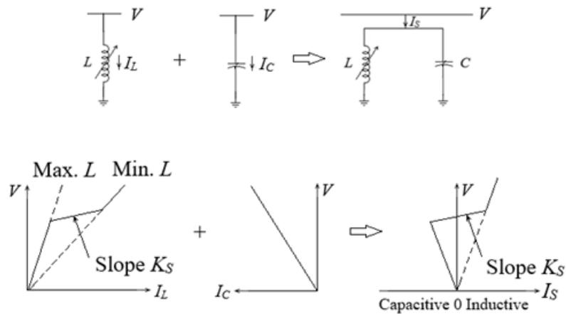
Figure 3.3. – Composite characteristics of an SVS[62].
