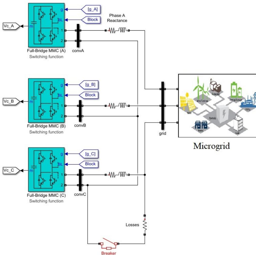
STATCOM (Detailed MMC Model with 22 Power Modules per Phase)
