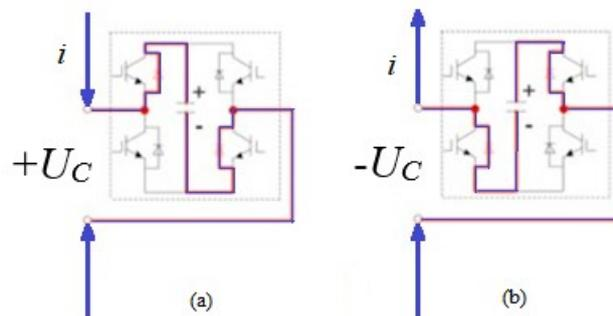
Figure 6.4.2. – Current path in full-bridge. (a) when the current is in the positive direction; (b) when the current is in the negative direction.
