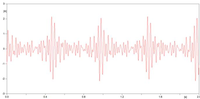
Figure 6.5.3. – Wind turbine harmonic current.
