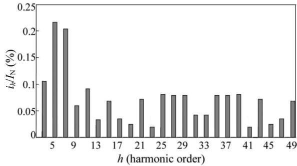
Figure 6.6.2. – Current harmonic distortion spectrum.
