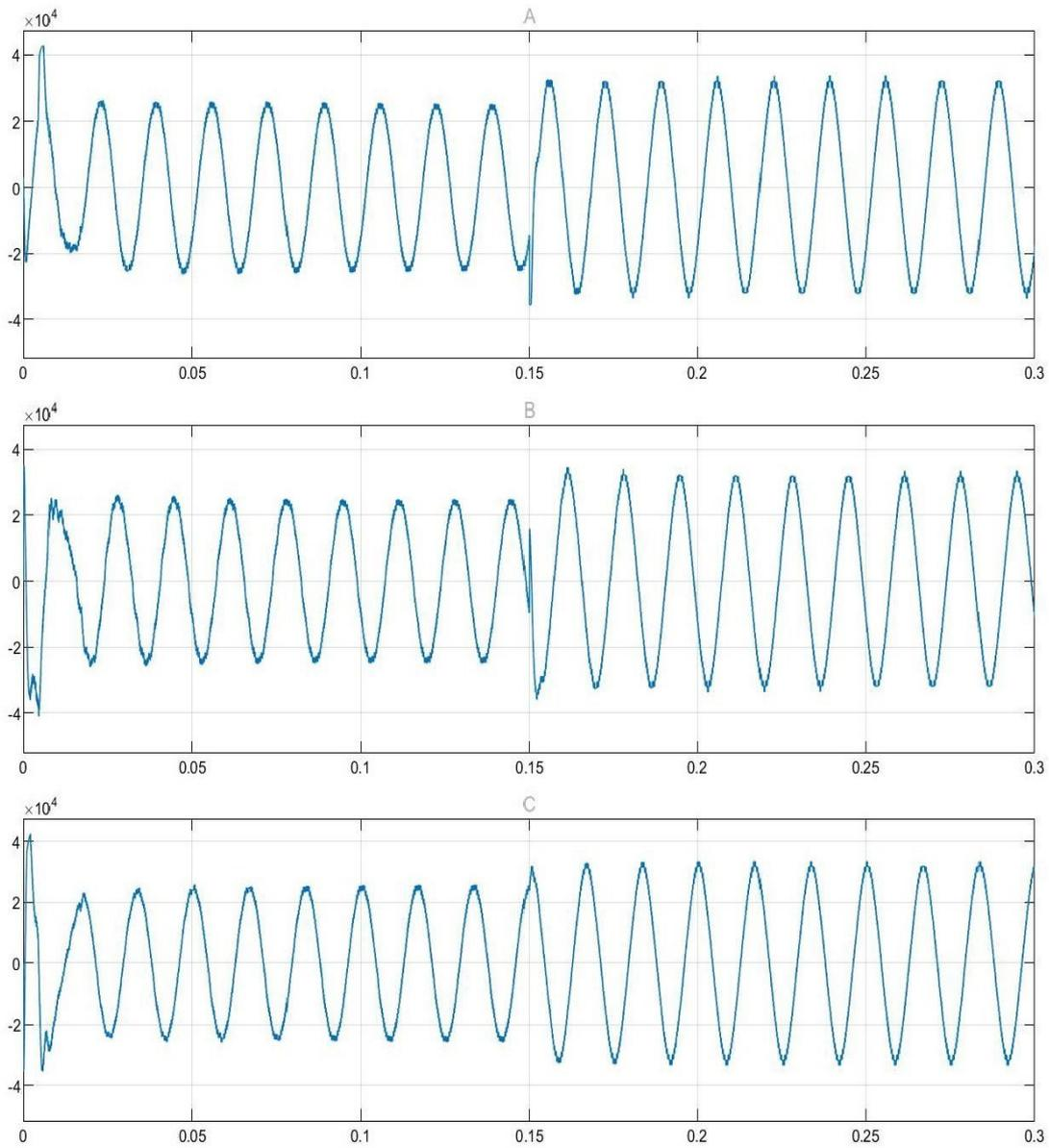
Figure 6.4.6. – Voltages at the exit of the statcom.
