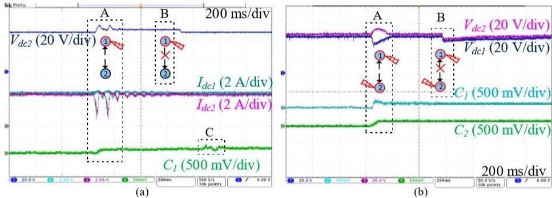
Figure 4.1. – (a) Experimental validation and (b) stealth attack on the voltage sensor (s) in a DC microgrid with  $M = 2$  agents [71].
