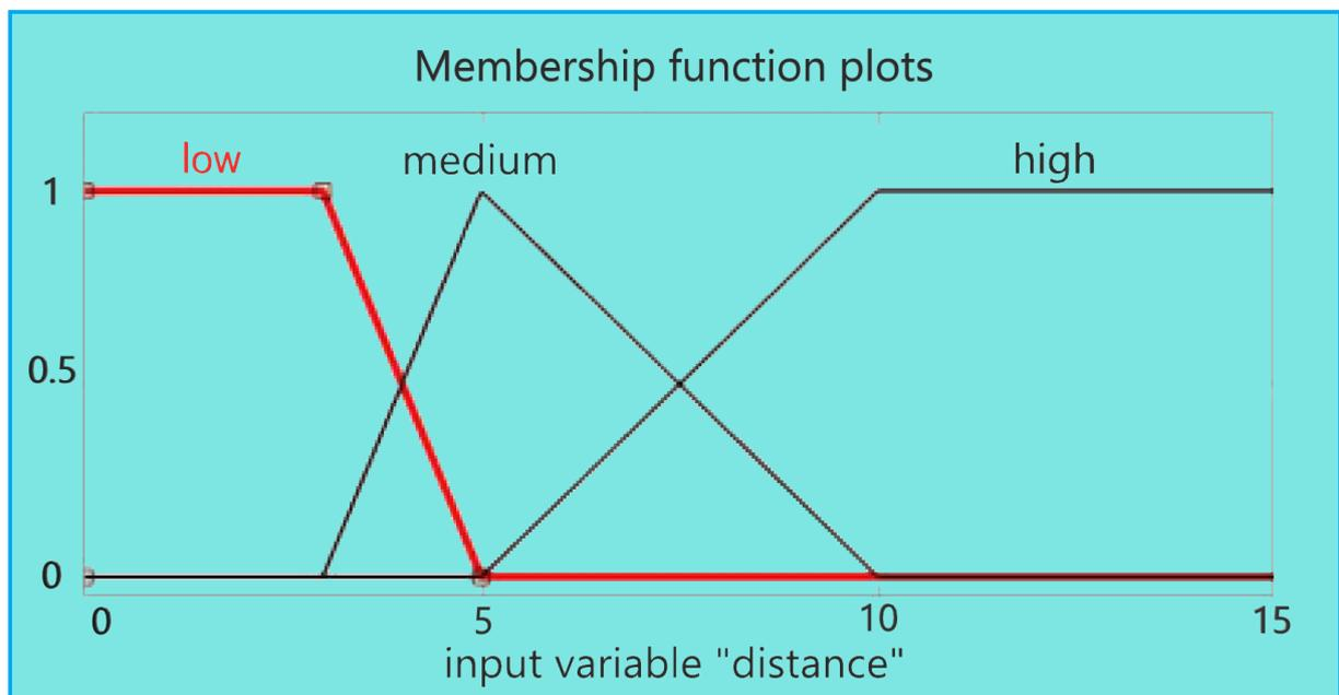
Figure 6.1.3. – Input variable Distance.
