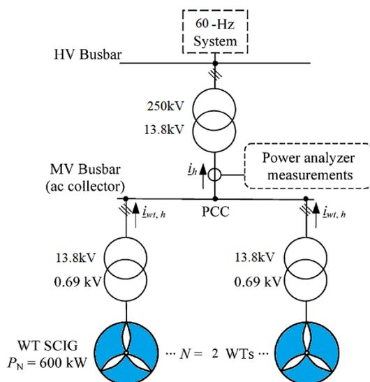
Figure 6.5.1. – Wind Turbines connected to the distribution system.
