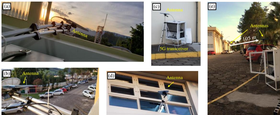
Figure 5.4 – Photographs of the FiWi system implementation in outdoor environment: (a) and (d) The transmitting antenna; (b) The wireless link view from RRU; (c) The 5G transceiver; (e) The wireless link view from the receiver side.
