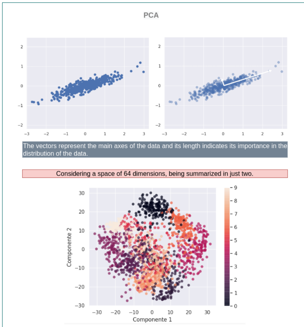
Figure 2.23 – A 64-dimensional space with 128000 is reduced by PCA to just two dimensions containing 4000 points.
