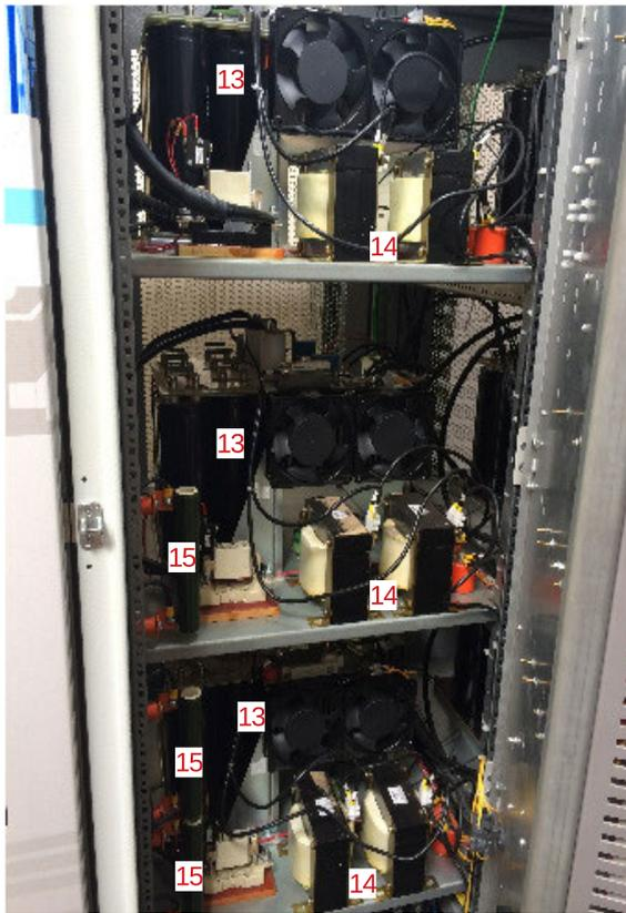
FIGURE 15. Power subsystem (of one phase).
