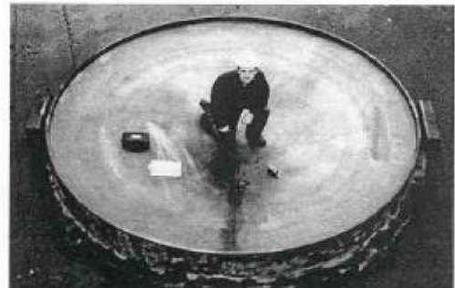
Concave for Benicia-Martinez Bridge Bearing
