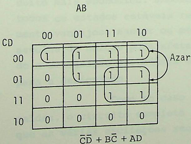
$\bar{C}\bar{D} + B\bar{C} + AD$
