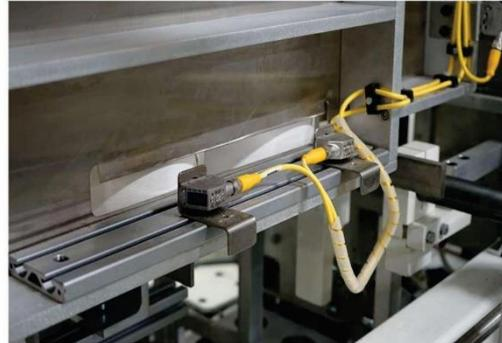
Fig. 11. Photoelectric IO-Link sensors in an EDSON packaging machine.
