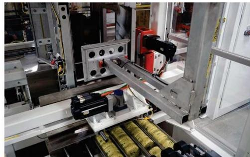
Fig. 12. Photoelectric IO-Link sensors in an EDSON packaging machine.
