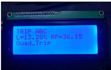
Figura 69 – Display LCD 20x4
