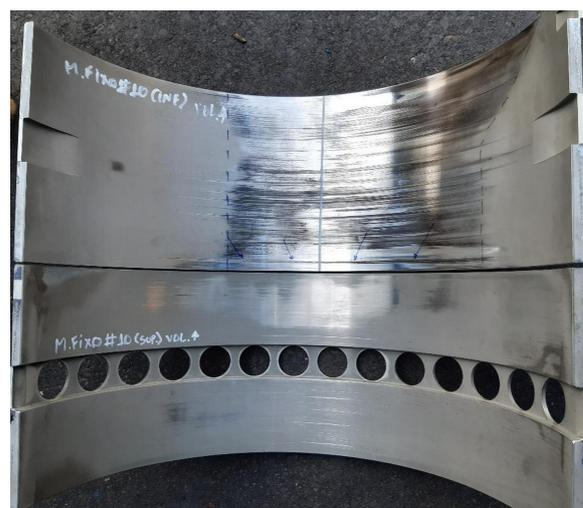
**Figure 13.** Photography of one of the disassembled bearing shells.
