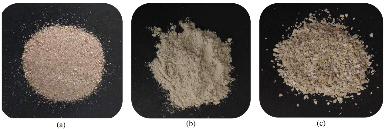
Figure 3-1: Fine aggregate used in the mortar: (a) River sand; (b) Polyurethane residue MF equal to 1.9; (c) Polyurethane residue MF equal to 3.1.
