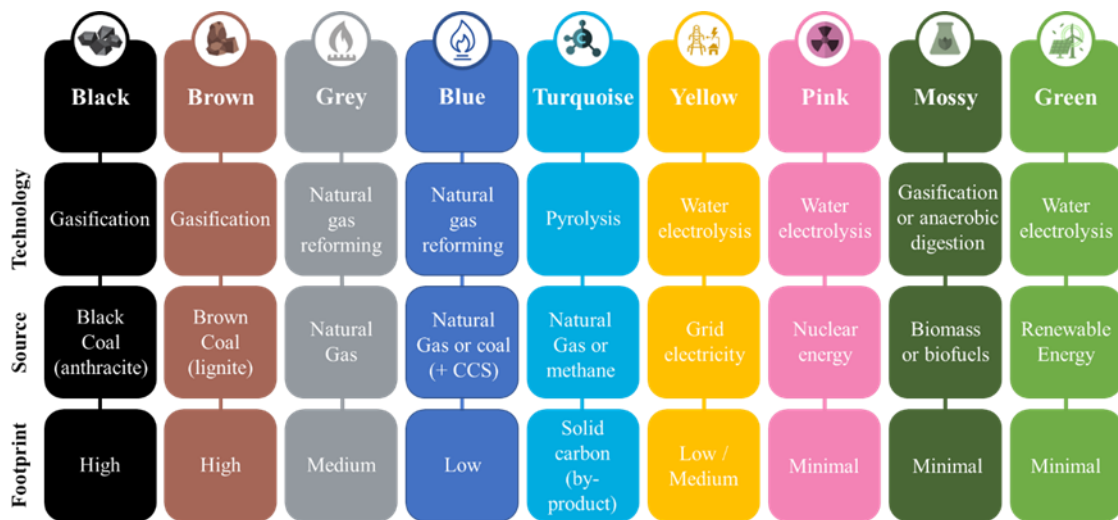
Fig. 2.2. Classification of hydrogen in a color scale.
