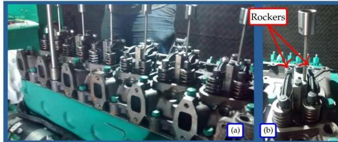
**Figure 6.** In-cylinder pressure tubes installed at the cylinder head—(a) general view—(b) zoom of one of the cylinder tubes.
