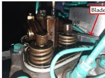
Figure 25. Simulated failure of loose clearance at the inlet valve of Cylinder 06.
