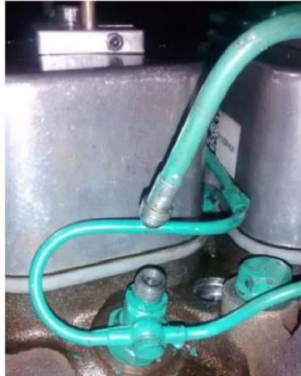
**Figure 19.** Simulated failure at the fuel injection of Cylinder 06.
