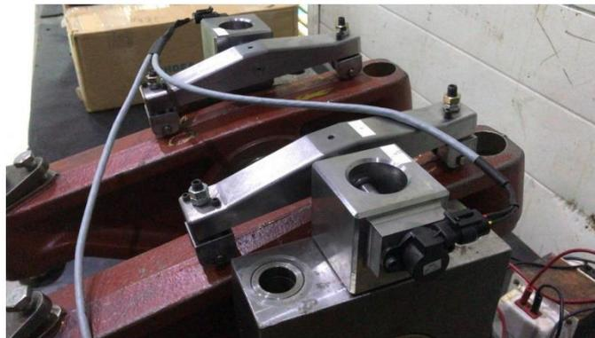
**Figure 14.** Resistive sensors installed at the rocker arms.
