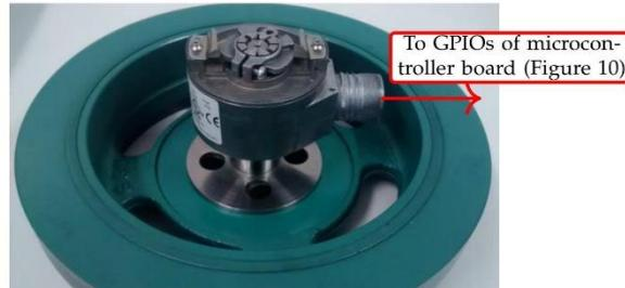
**Figure 12.** Encoder installed on the crankshaft pulley disk.
