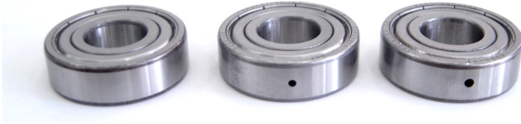
Fig. 1. Tested bearings (from left to right): healthy, fault #1, and fault #2.
