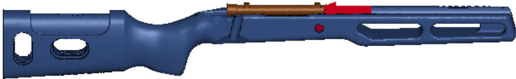
Figure 5.10 – Red arrow indicating the region of application of the ammunition pressure curve on the bolt face.
