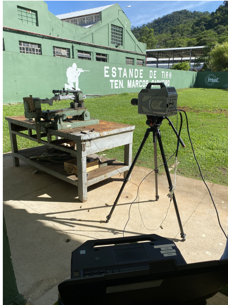
Figure 5.4 – Experimental setup, in which the firearm mounted on the test stand can be observed, along with the high-speed camera positioned perpendicular to the firearm axis and connected to a computer for storing the acquired images.
