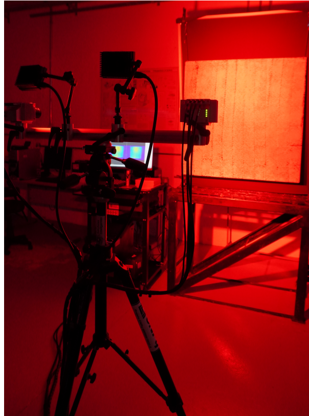
(a) Experimental setup for modal testing using DIC and electrodynamic shaker.
