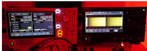
(b) Time-domain representation of the swept-sine excitation signal monitored using a digital oscilloscope.
