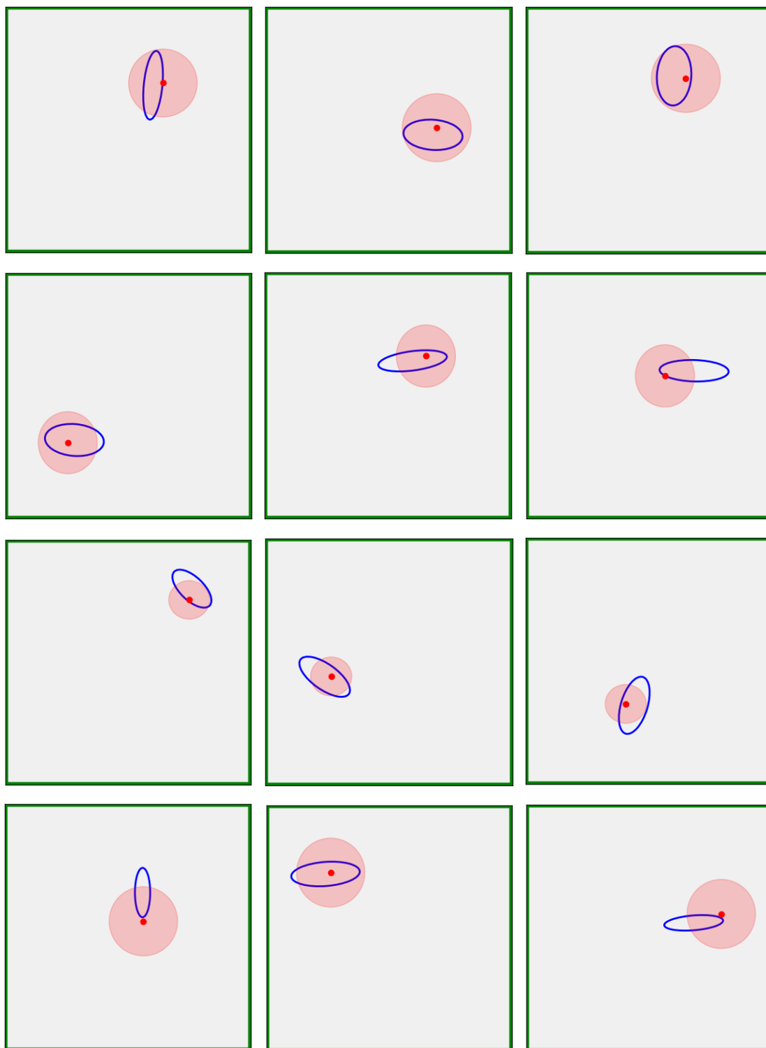
Figure 3.11: Core Damage location: Line 1 - FFFF; Line 2 - CFFF; Line 3 - CCFF; Line 4 - CCCC. Legend: \circ Real damage \bullet Predicted position of the damage \odot 95% confidence interval.
