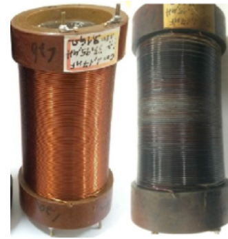
Fig. 6. Test sample before (left) and after (right) several sessions of thermal stress.
