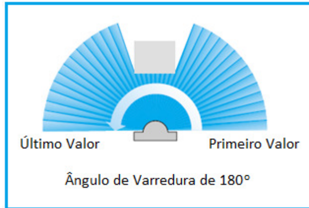
Figura 4.2 - Leque de varredura do scanner laser .
