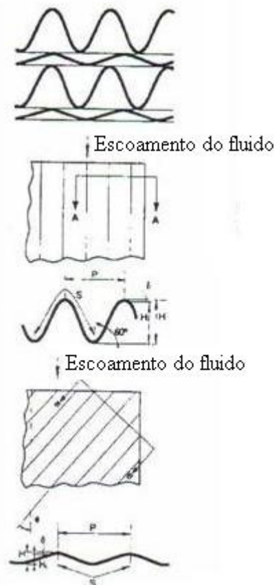
Figura 3.17 – Superfície “Corrugated Undulated Surface” (Utriainen e Sundén, 2002)
