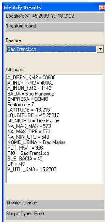
FIGURA 7.34 – Características hidráulico – operativas da UHE Três Marias (Fonte: ESRI ArcExplorer™ (1997). A GIS data explorer built with MapObjects™ technology. Disponível em: [http://www.esri.com/software/arcexplorer/index .html](http://www.esri.com/software/arcexplorer/index.html); Environmental Systems Research Institute, Inc.)
