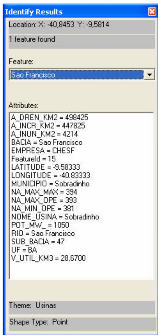
*FIGURA 7.31 – Características hidráulico – operativas da UHE Sobradinho (Fonte: ESRI ArcExplorer™ (1997). A GIS data explorer built with MapObjects™ technology. Disponível em: [http://www.esri.com/software/arcexplorer/index .html](http://www.esri.com/software/arcexplorer/index.html); Environmental Systems Research Institute, Inc.)*
