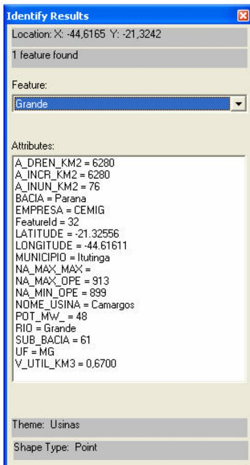
*FIGURA 7.8 – Características hidráulico – operativas da UHE Camargos (Fonte: ESRI ArcExplorer™ (1997). A GIS data explorer built with MapObjects™ technology. Disponível em: [http://www.esri.com/software/arcexplorer/index .html](http://www.esri.com/software/arcexplorer/index.html); Environmental Systems Research Institute, Inc.)*
