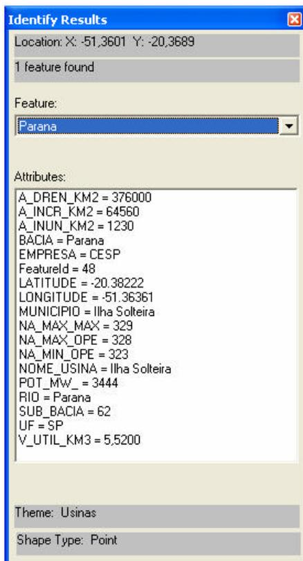
FIGURA 7.20 – Características hidráulico – operativas da UHE Ilha Solteira (Fonte: ESRI ArcExplorer™ (1997). A GIS data explorer built with MapObjects™ technology. Disponível em: [http://www.esri.com/software/arcexplorer/index .html](http://www.esri.com/software/arcexplorer/index.html); Environmental Systems Research Institute, Inc.)
