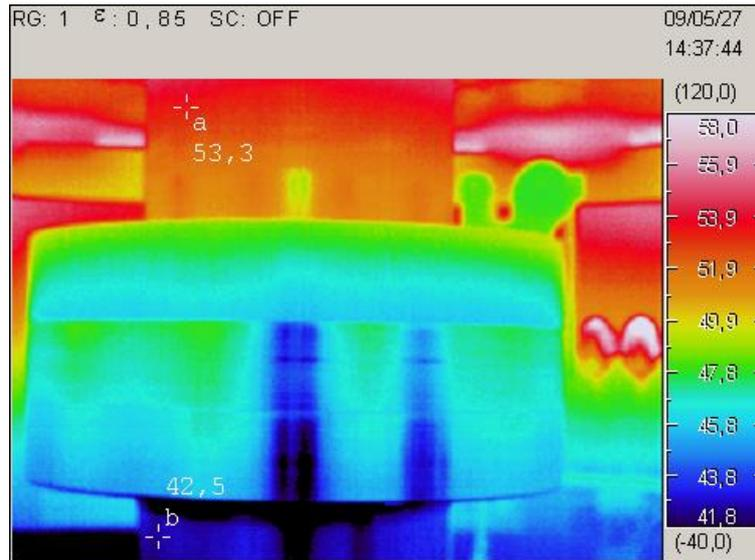
Figure 4.7. IR thermal image of a generator shaft.
