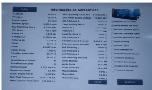
Figure 10. Picture of a PLC hub web browser access screen of unit #25.
