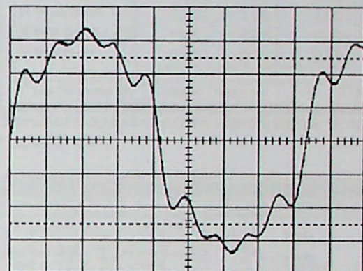
Actual output waveform from HGA controlled AC i-Series power system
