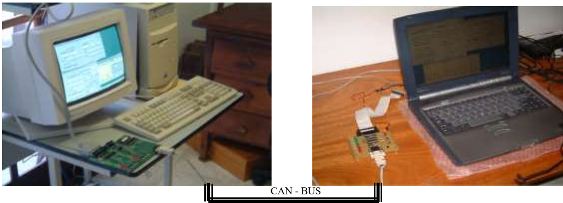
Figura 8.3-Conexão PC transmissor com PC receptor
