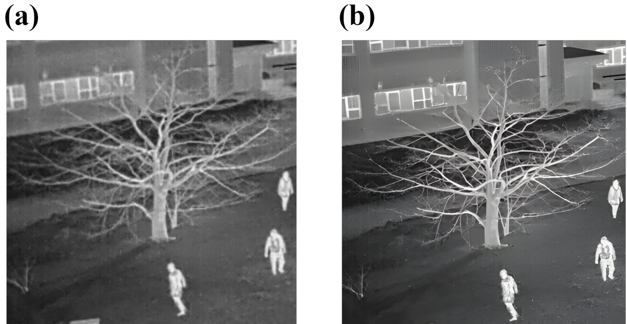
Figure 5 – Example of satisfactory contrast enhancement in image resolution by Real-ESRGAN. (a) Image before enhancement. (b) Image after the process.
