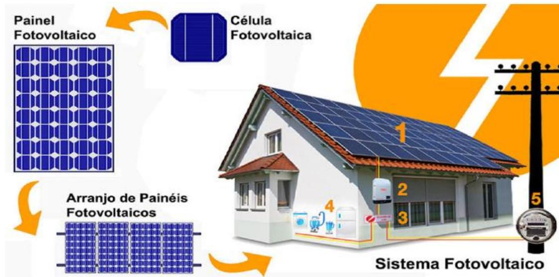
Figura 6: Sistema on-grid.
