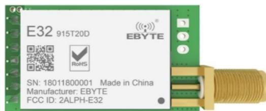
Figura 13 – Modulo transmissor LoRa E32-915T20D, figura do autor.
