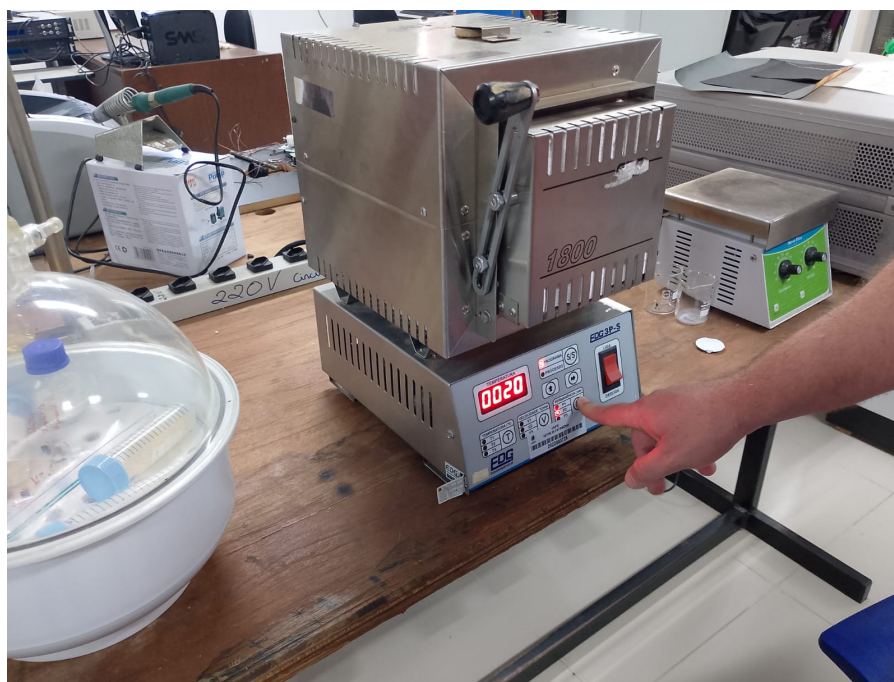
Figura 8 – Forno FDG 3P-S com as amostras a 900°C.
