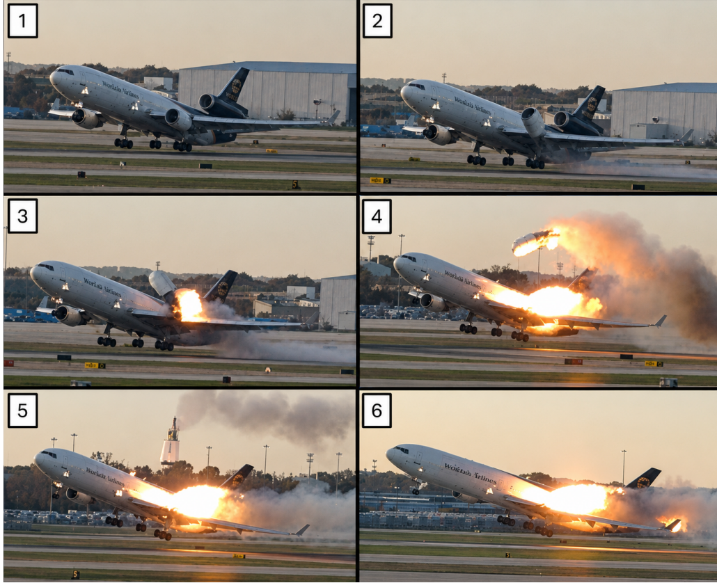
Figure 5.1 – Surveillance footage sequence illustrating the catastrophic separation of the left engine and pylon from the wing of the UPS Flight 2976 MD-11F aircraft shortly after takeoff (adapted from (14)).
